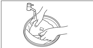
Wash the Filter in water by hand. (Do not use washer or dryer).
