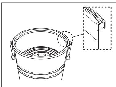
Please ensure to place the Filter Supporter to its original location in order to avoid Filter Supporter become deform which can cause dust leakage.
