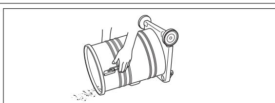
Remove the Filter and empty dirt and dust.
