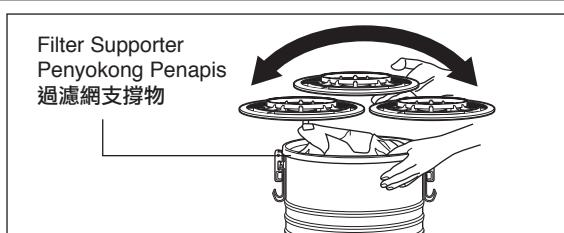
Hold the Filter Supporter and pull the Expander upward and shake it about ten times. (Never shake up and down while Hose connected.)
