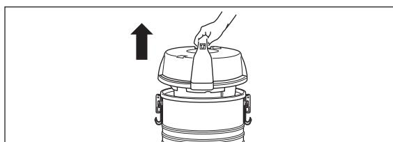
Remove the Motor Housing hanging upward with the Carrying Handle.
