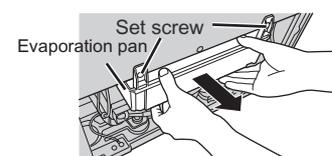
Removing the screw, then hands hold the Evaporation pan slowly pull out.
