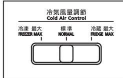
Usually, use this refrigerator with this cold air volume-adjusting lever set to "標準 Normal". If the freezer compartment or the refrigerator compartment isn't cooled sufficiently, you can adjust the cold air volume.
