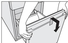
Lift it up slightly and pull it out onto the ground.
