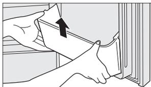
Remove with a light tap from below (it is firmly secured) .
