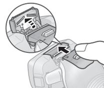
Press and hold the top knob (a) and slide the trimmer handle down to lower the trimmer.
