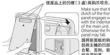
Make sure that the clutch of the front panel engages well with the indentations of the main unit. Otherwise the front panel may fall.
