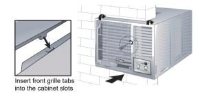
8 Attach air filter to the front grille. (see Anti-bacterial filter installation instructions included in this package)
