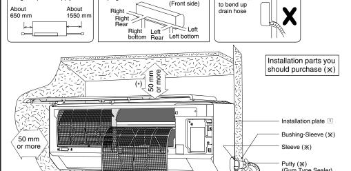
Putty (※) (Gum Type Sealer) Bend the pipe as (Left and right are identical) closely on the wall as possible, but be careful that it doesn't Insulation of piping connections Carry out insulation after Power supply cord (X) checking for gas leaks and secure with vinyl tape. Vinyl tape (wide) (X) X Vinyl tape Apply after carrying out a drainage test. To carry out the (Attaching the remote control holder to the wall) drainage test remove
